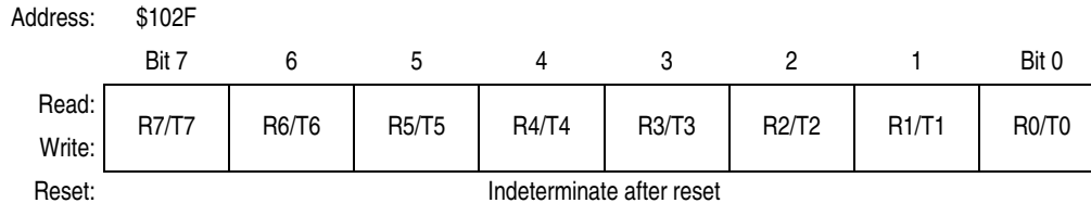
Figure 7-3. Serial Communications Data Register (SCDR)
